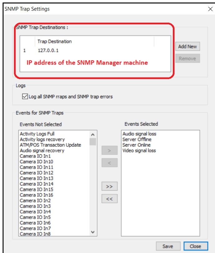
**SNMP Trap Destinations:** user can specify the IP addresses of SNMP Manager applications which will receive the traps for selected events.
